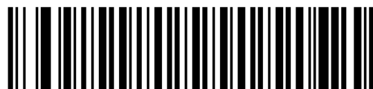
Quick multiple-prefix example: AB (ASCII values: 0x41 and 0x42)
