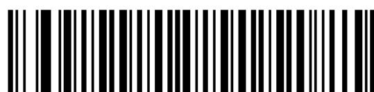
Quick multiple-suffix example: AB (ASCII values: 0x41 and 0x42)
